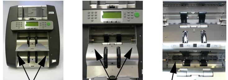
Stacker 2 release latches (Fig 1)      Location posts / slots (Fig 2)      Note diverter (Fig 3)
