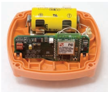
Figure 10: StatusCheck End Node Battery Orientation
