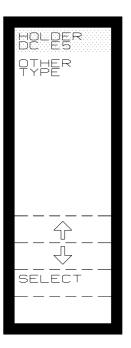
Select another sprayer type by pressing "SELECT TYPE" then move the cursor to the required type and press the "SELECT" key.
