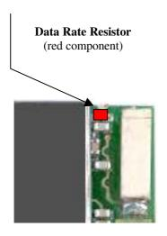
The purpose of this resistor is to be able to access the ARF32 module by forcing the UART data rate in case of bad "Non Volatile Settings" programming during test and evaluation.
