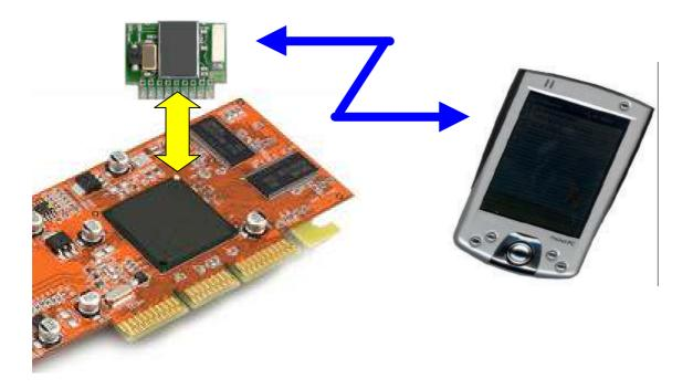
The ARF32 module full complies with the V1.1 Bluetooth<sup>®</sup> standard and data rate goes up to 723 kbps. Data exchange and set-up are only done through an UART data port, under SPP profile. Miniature antenna is integrated.
