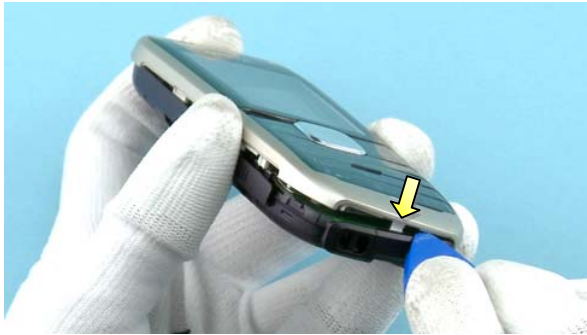
7) Release the clip on the bottom side of the A-COVER ASSY.
