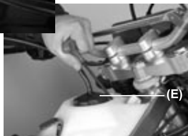
6. Unscrew screw of fuel tank (E).
