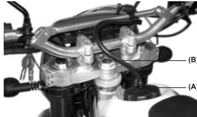
(A). Fuel Cap. (B). Fuel Vent hose.
