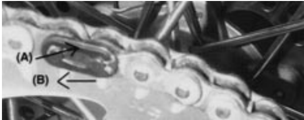
(A). Clip. (B). Direction of Chain Rotation.
