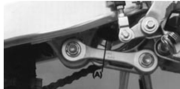
(A). Rebound dampening adjuster
