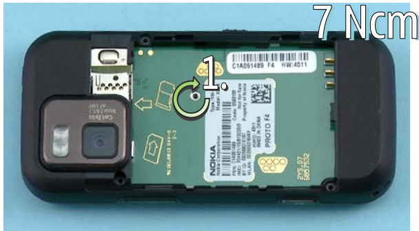
7) Tighten this M1.2X2, PANHEAD 2.5X0.6 T PLUS-4IP screw to the torque of 7 Ncm.
