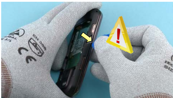
9) To release the B-COVER close the slide and insert the SRT-6 between the hinge assembly and the B-COVER. While detaching the B-cover, be careful not to touch the engine board.
