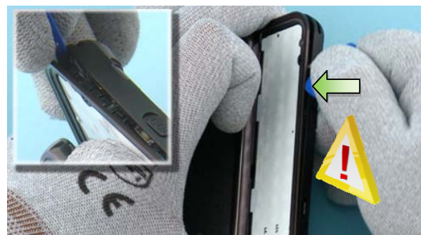
12) Carefully slide the phone open. Use the SRT-6 to release the remaining clips holding the B-COVER. Remember not to touch the engine board.
