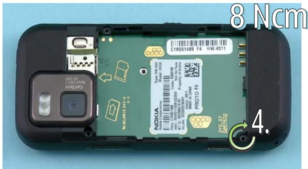
9) Tighten this M1.4x2.5 TORX PLUS-4IP screw to the torque of 8 Ncm.
