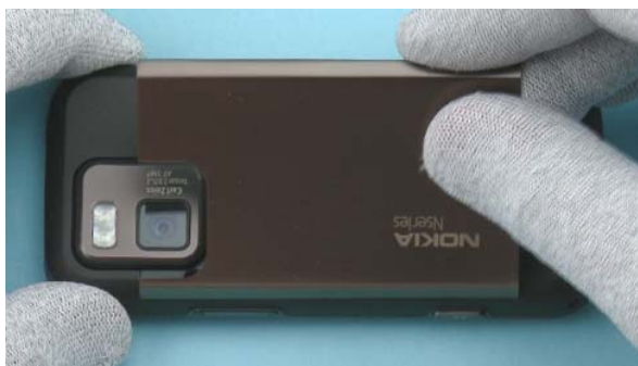
11) Make sure the battery cover is assembled correctly. First attach the hooks on the Camera/Volume key side. Then close the LOCK KEY side.
