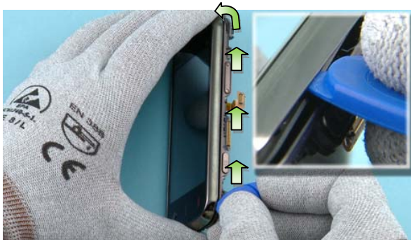
29) Start releasing the A-cover assembly with the SRT-6 as shown.
