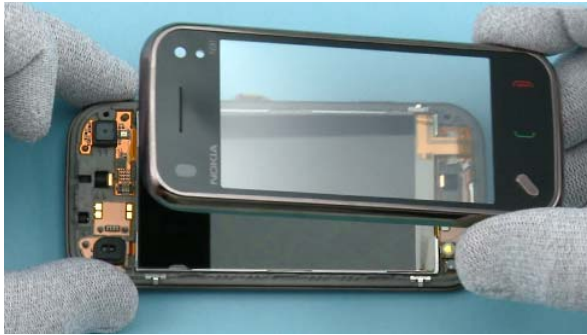
31) The A-COVER can now be separated.
