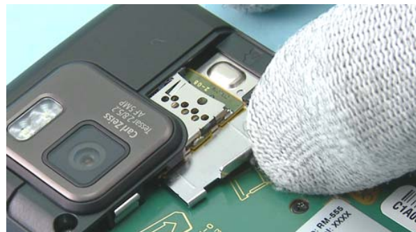
10) Insert the USIM CARD TRAY.
