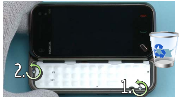
8) Unscrew the two TORX+ size 4 screws in the order shown. Discard the screws.
