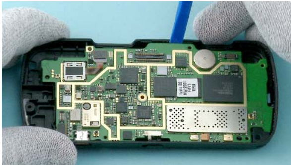
21) Release the engine board with the SS-93.
