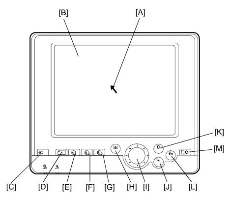
The scanned image is sent to the display editor and displayed on the LCD ( $640 \times 480 \text{ dot}$ ).
