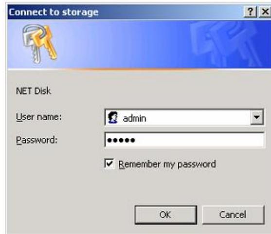
When two new NASs are simultaneously connected to your network, you need to distinguish between the two by typing “http:// Storage-XXXX” with their unique MAC address. Please refer to the sticker on the rear panel for the address and replace XXXX with the last four digits of the MAC address.
