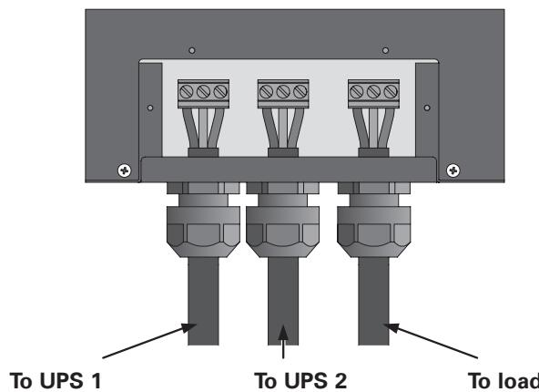
1. Connect input power cables to two UPSs (UPS1 (S1) is the preferred source).
