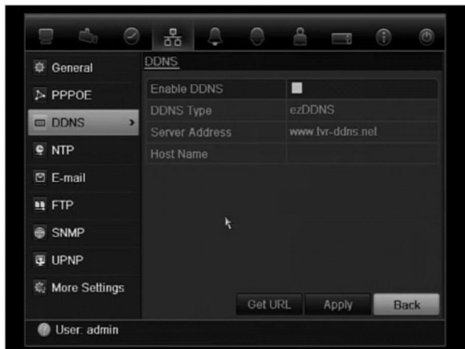
Figure 34: ezDDNS setup window
