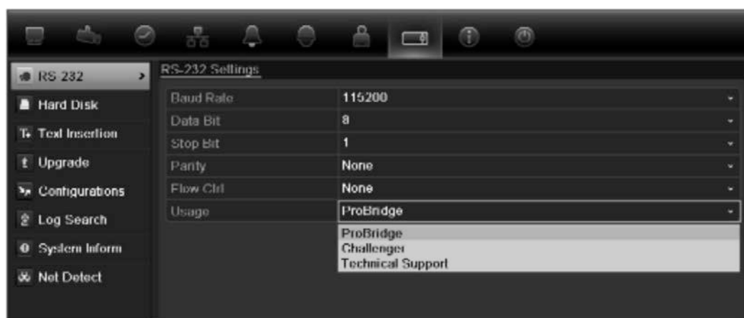
Figure 38: RS-232 setup window
