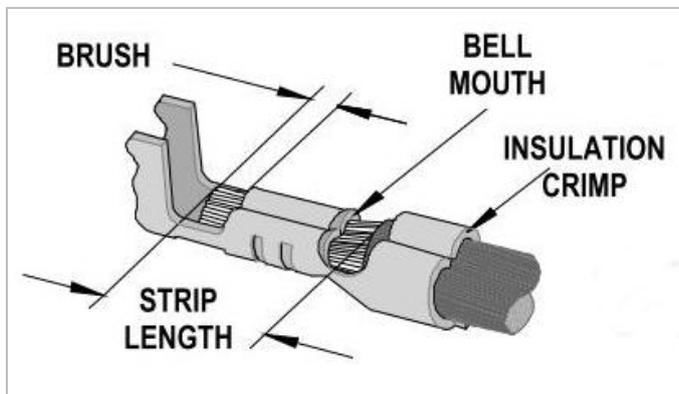
**Figure 3-1. Stripped Wire in Crimp Pin**
