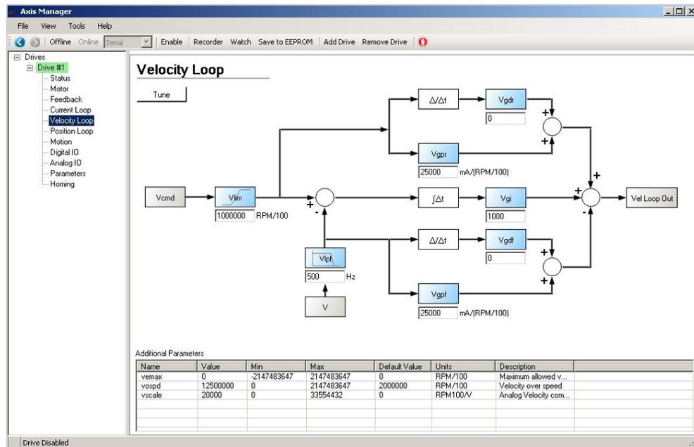
**Figure 4-17. Velocity Loop Parameters Screen**
