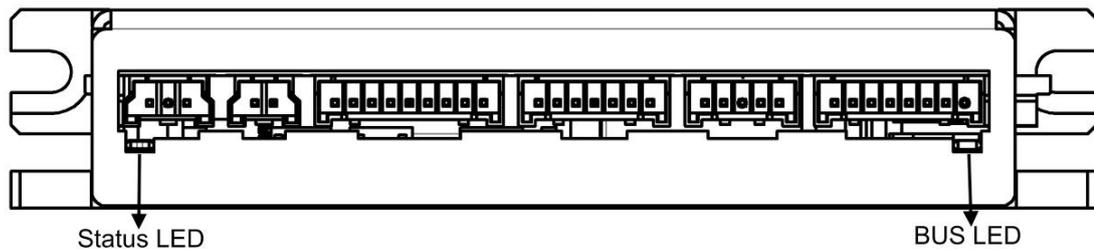
**Figure 3-17. LED Indicators on Front Panel**
