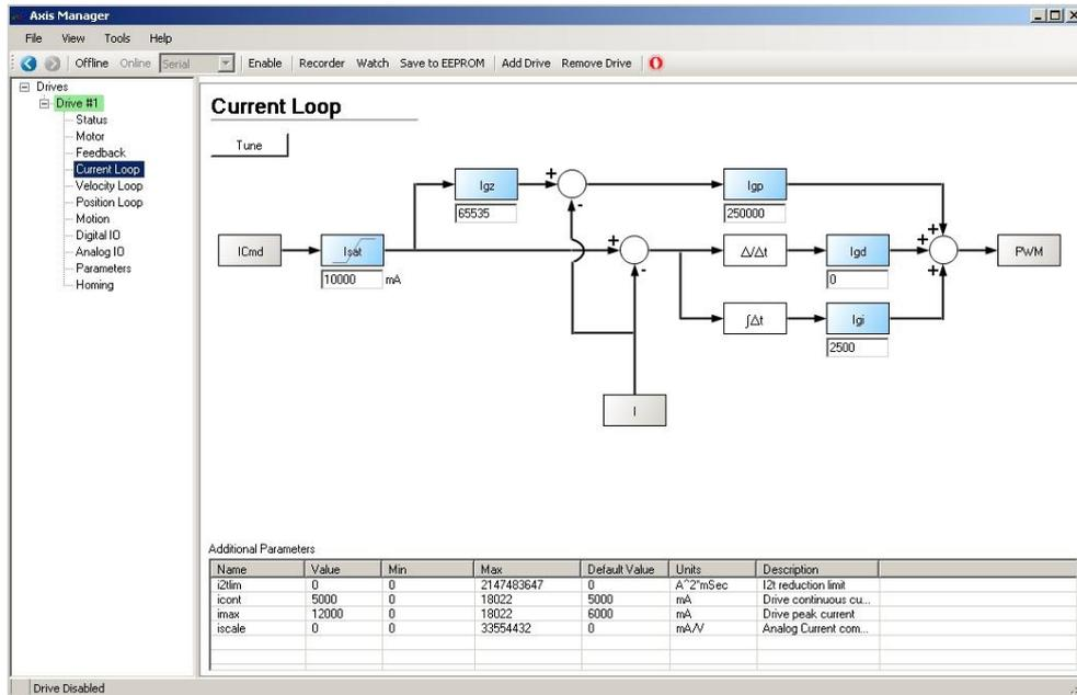
**Figure 4-16. Current Loop Parameters Screen**
