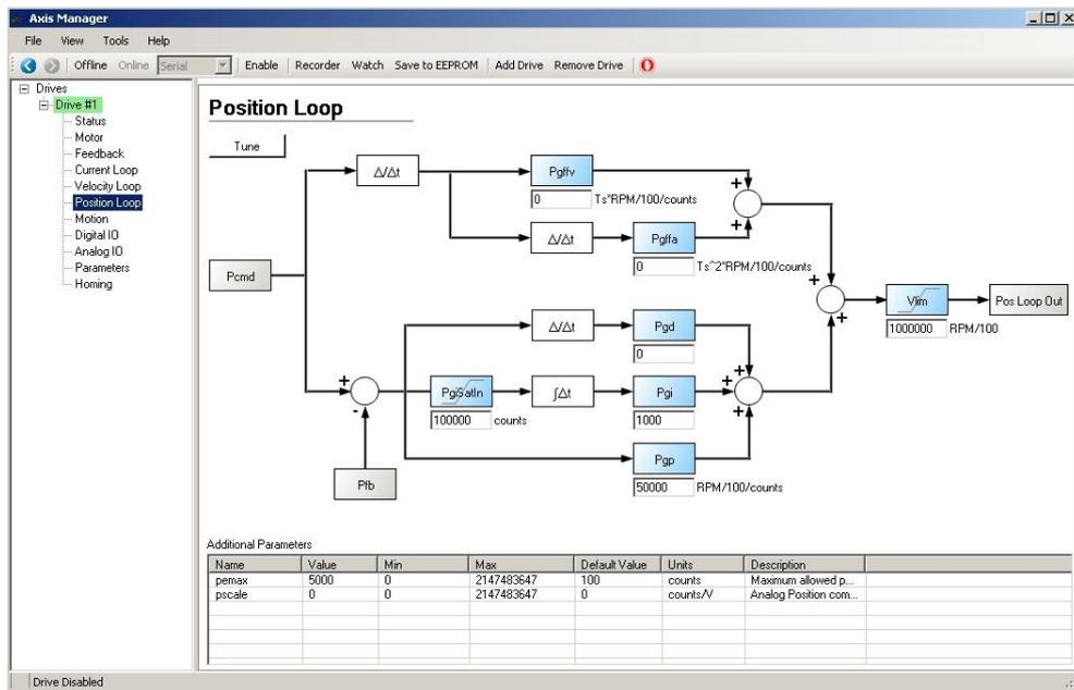
**Figure 4-18. Position Loop Parameters Screen**
