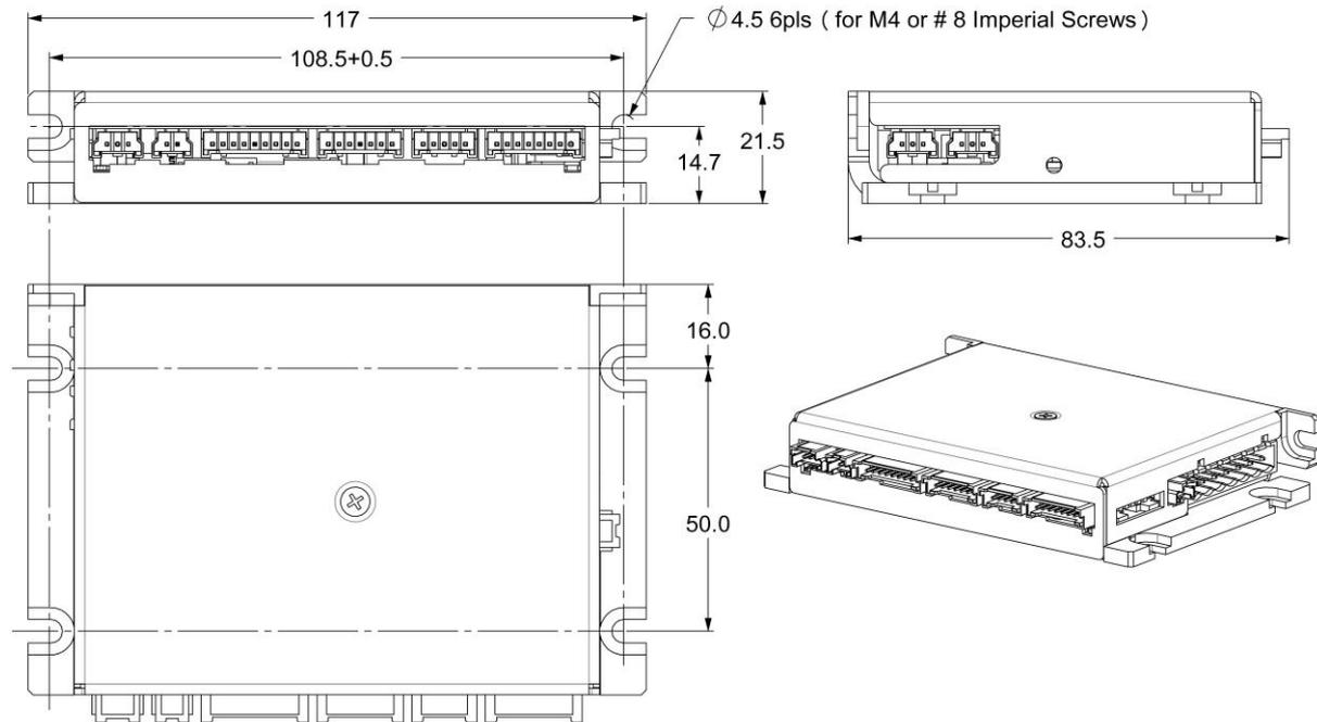
**Figure 3-2. LVD Dimensions and Mounting Holes**
