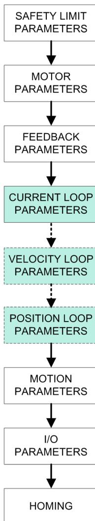
**Figure 4-12. Drive Parameter Configuration Sequence**
