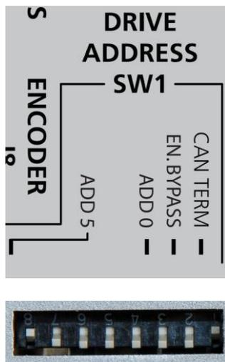
**Figure 3-16. DIP Switches**
