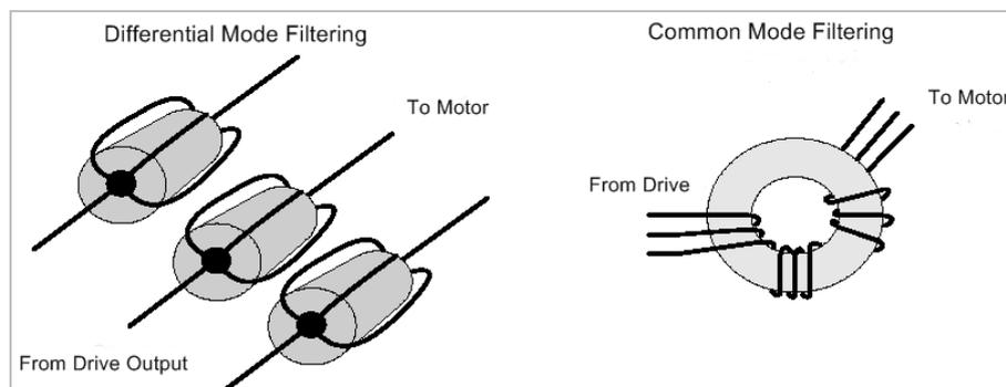
**Figure 3-3. Mode Line Filtering**
