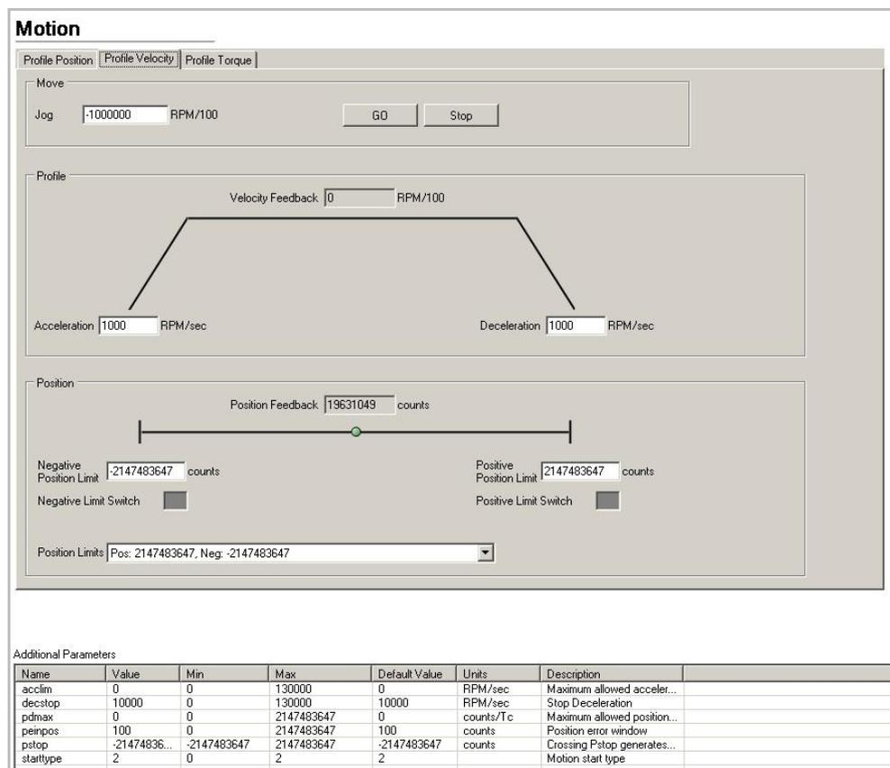
**Figure 4-20. Motion Screen – Velocity Profile Tab**
