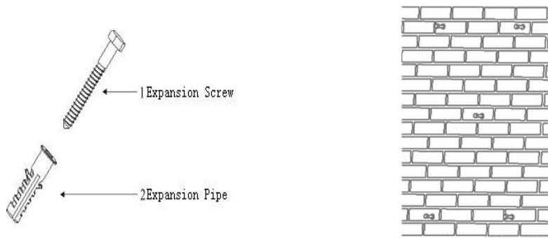
Figure 9 Installation of Expansion Pipe
