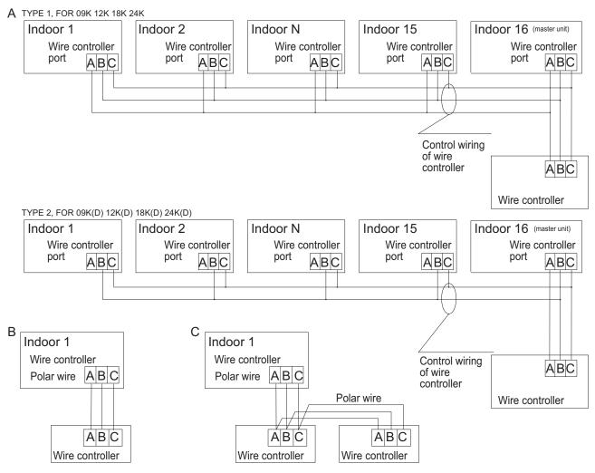
There are three methods to connection wire controller and the indoor units:
