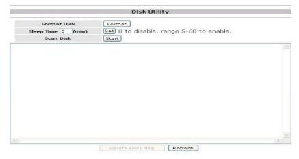
Since the LanDrive supports power management, you can also determine the time the hard drive have to be inactive in order for the LanDrive to enter sleep mode. The Scan Disk function can be used to detect potential problems with the hard drive. Click on the refresh button to display the scandisk result.
