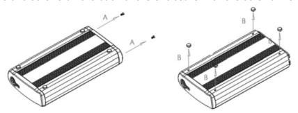
**B.** Loosen the four screws on the surface of the unit. These screws willbe used later to minimize the gap between the heat sink and your hard drive
