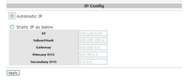
The LanDrive can also act as a DHCP server when one is not present in your network. The default IP of the LanDrive in DHCP server mode is "169.254.0.1" and any device that is linked to the network containing will be assigned an IP of "169.254.0.x" automatically.
