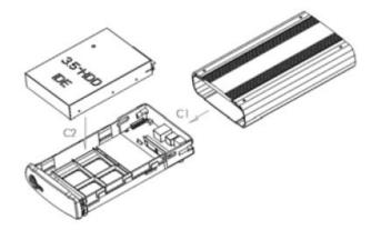
**C.** The plastic brackets should slide out effortlessly. Inster your hard drive, connect the IDE and power cable from the enclosure accordingly.
