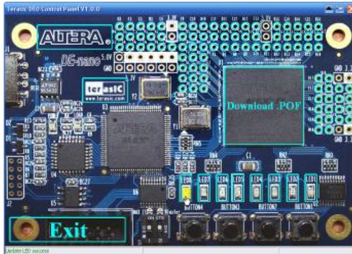
Figure 3.4 Control panel window for LED controlling.
