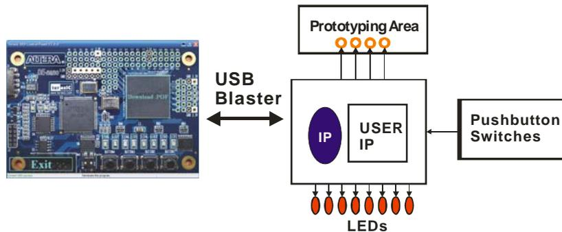
Figure 3.3. The MAX II Micro Control Panel concept.
