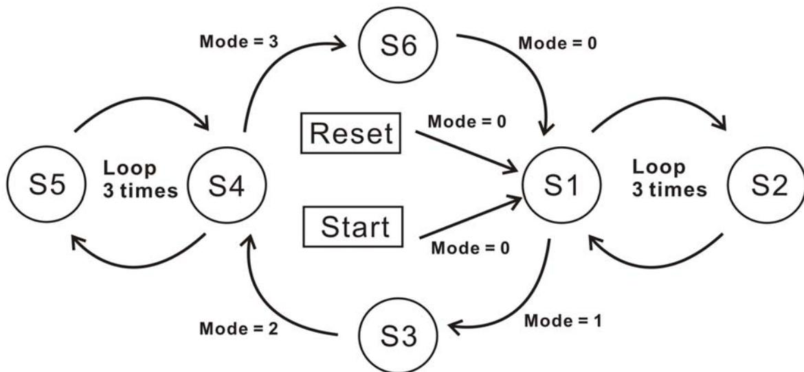
Figure 4.2 State flow chart of traffic light.
