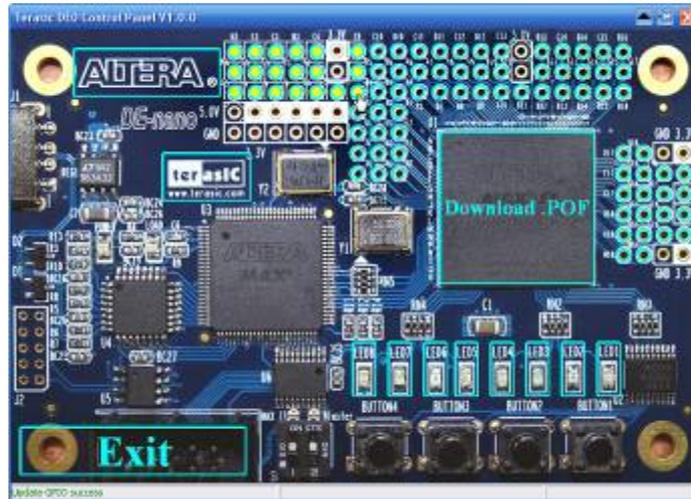
Figure 3.6 Users can configure the GPIOs in the prototyping areas by clicking on the corresponding holes shown in the Control Panel window section. The GPIOs' color will be marked by yellow to indicate their voltage level is HIGH (3.3V).
