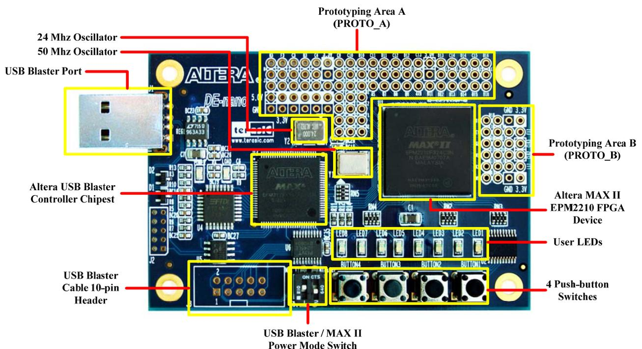
Figure 2.1. The MAX II Micro board.
