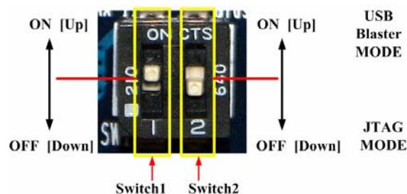
Figure 4.1. Set Switch1 to UP position and Switch2 to DOWN position in normal operation (JTAG mode)
