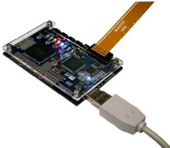
Figure 1.3. Connect to PC through USB cable.
