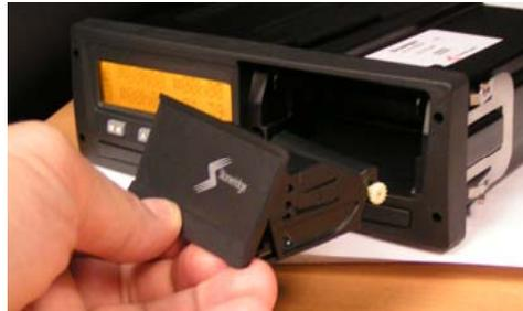
4. Gently pull the fascia mechanism forward out of the VU.
