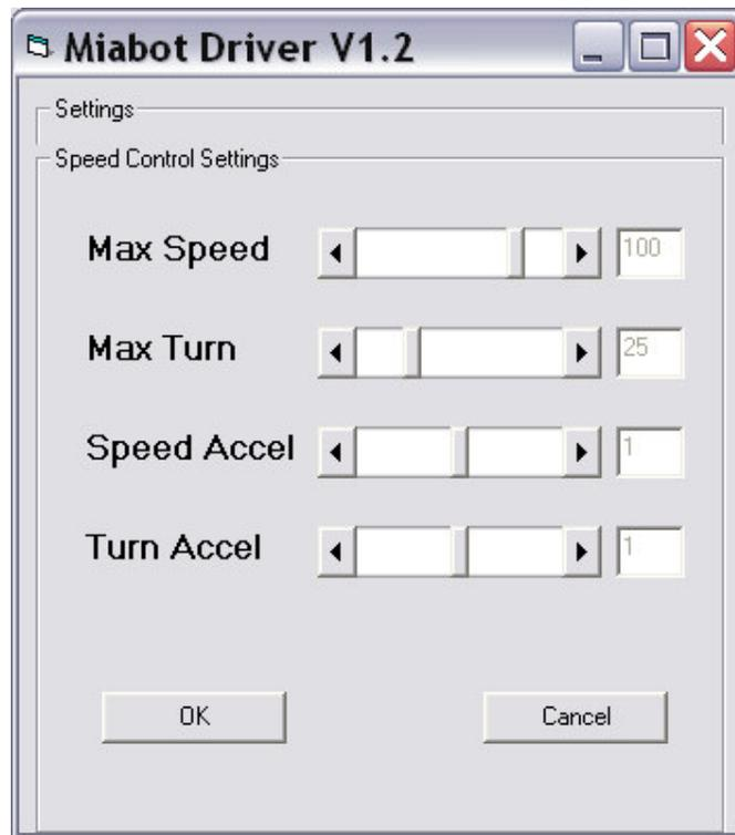
These sliders control the maximum speed and rate-of-turn applied to the robot (for full stick deflections), while the “accel” sliders adjust the speed of response.
