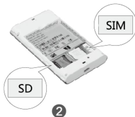
Refer to the above picture while install the SIM card, please open the battery cover first, insert the SIM card according to the direction of the arrow.
