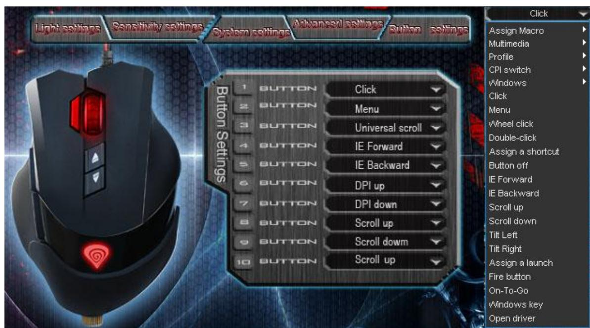
You can bind one of more than 40 functions to keys labeled by numbers on the schema above. In the right side of the window, you can see actual configuration of the buttons. Each position on the list is in fact a combo box, from which you can choose a preferred function for an individual button.
