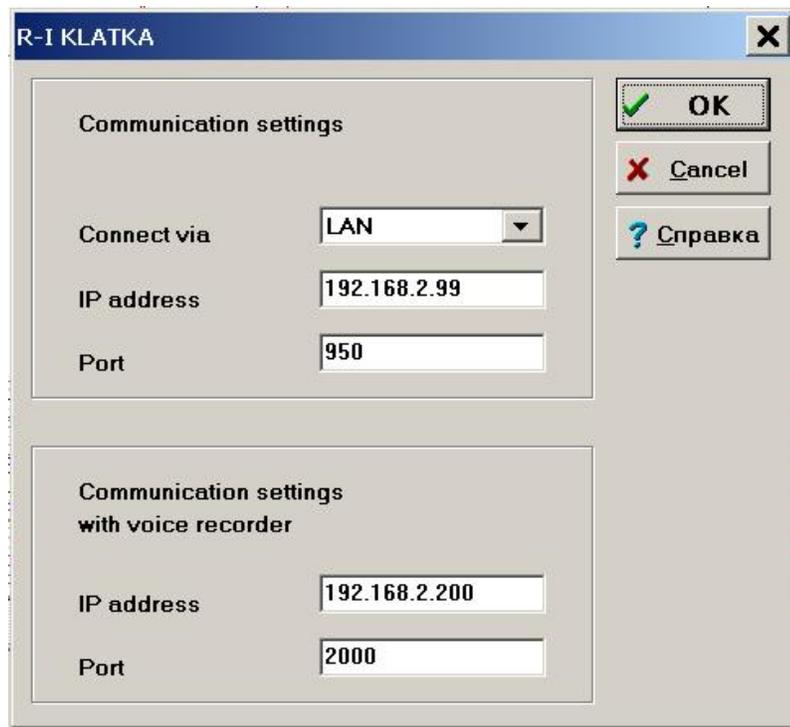
Figure 22.2: IP address and port number setting for voice recording
