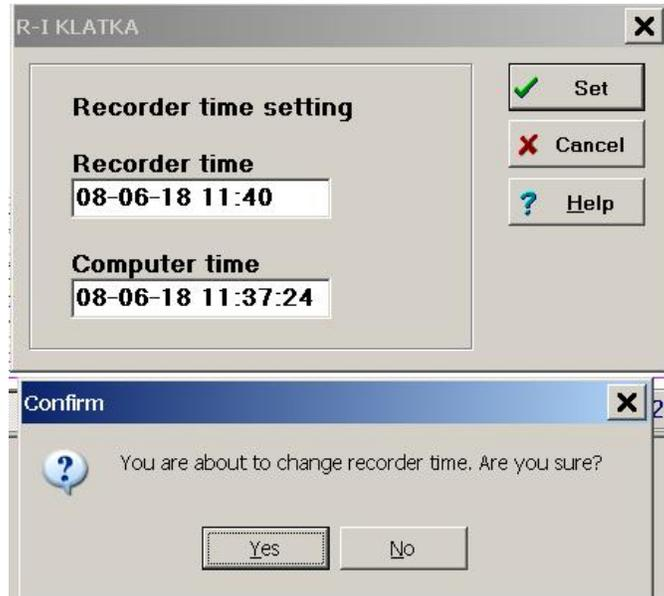
Figure 21.1: AR-2c datalogger time setting
