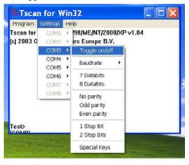
4. Set Baud rate to 9600, and 8 DatBits; No parity; 1 Stop Bit under COM3.
