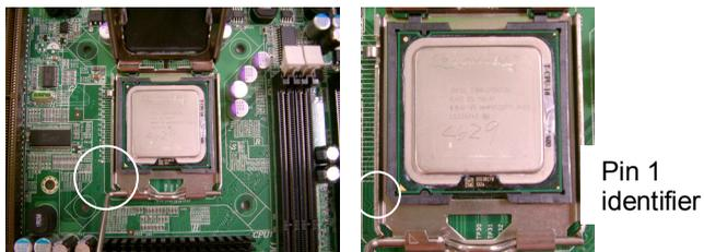
4. Remove the PnP cap from the load plate.
