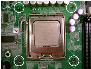
4. Press the heatsink down until the four screws are securely seated in the holes.
