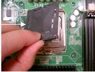
5. Replace the load plate and return the locking lever to the locking position.
