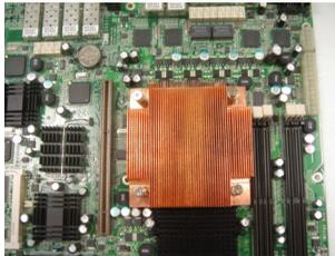
5. Use screw drive to secure the four screws.
