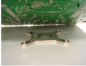
3. Align the heatsink with the four holes around the processor socket.
