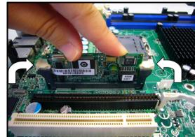
**NOTE:** The SO-DIMM expansion cards will fit in the slot only one way. Make sure that you align the slot in the card with the key in the card slot.
