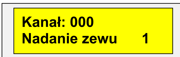
Illustration 17. Information in the display window when the key ZEW 1 is pressed.
