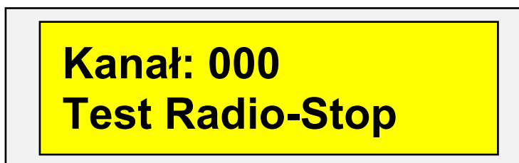
Illustration 15. Information in the display window after completion of the tests and switching to standard operating mode.
