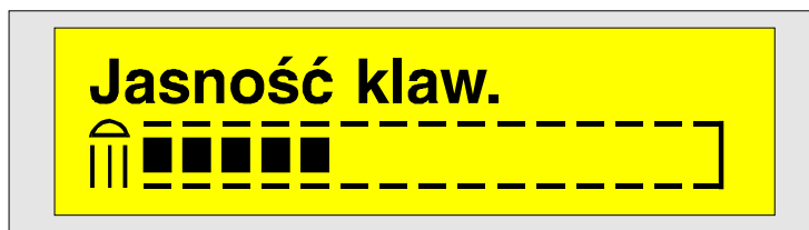
Illustration 26. Information in the display window during adjustment brightness of keypad illumination
