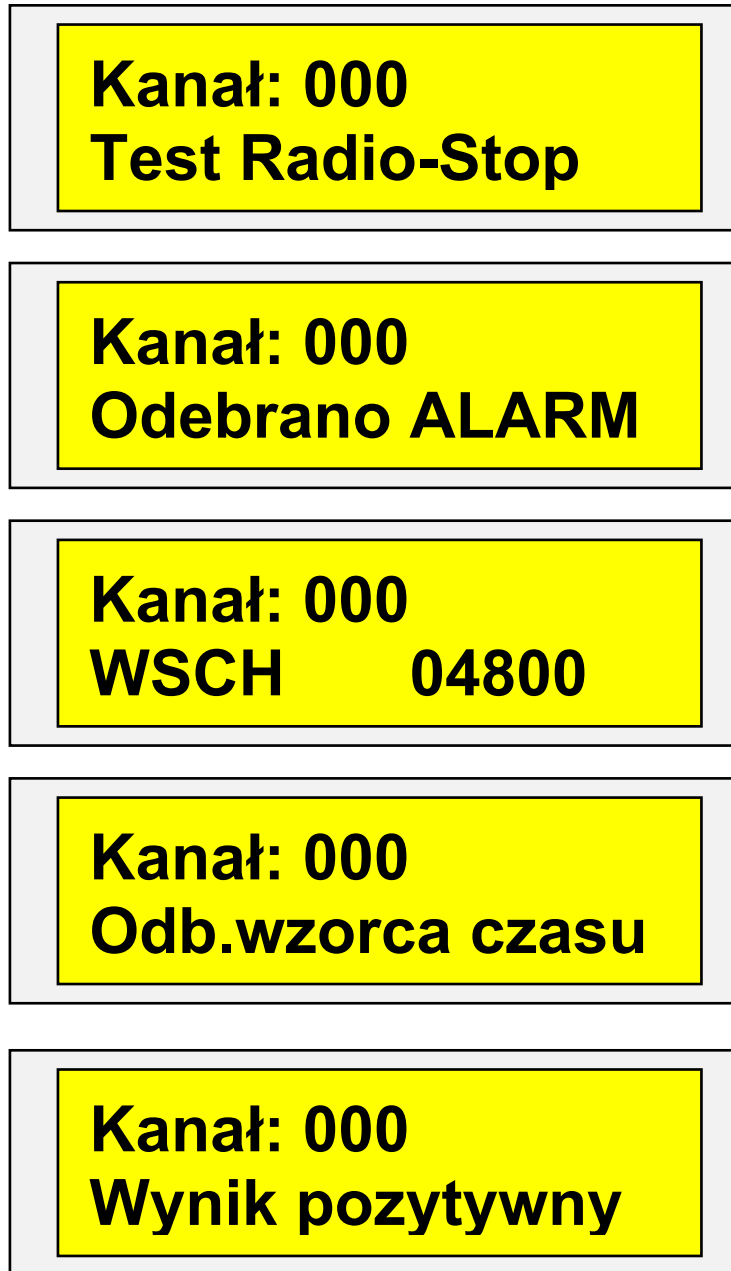
Illustration 53. Information in the display window during testing of the Radio-Stop system (correct result)
