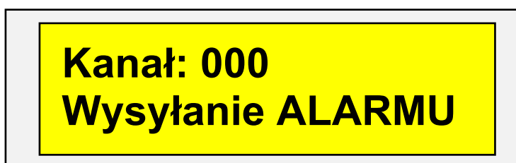
Illustration 16. Information in the display window during sending an alarm
