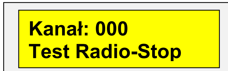
Illustration 56. Information in the display window after using the combination of keys F3+2
