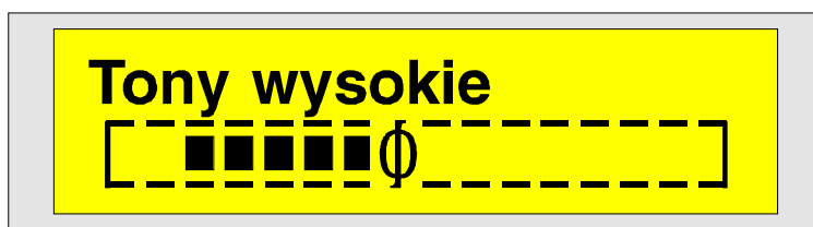
Illustration 29. Information in the display window during adjustment of high tones.
