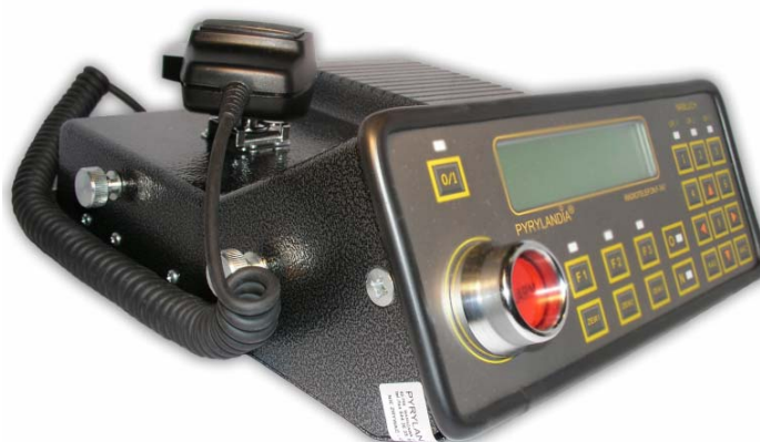
Illustration 3. View of the front plate of the control head F-747M (mobile version)
