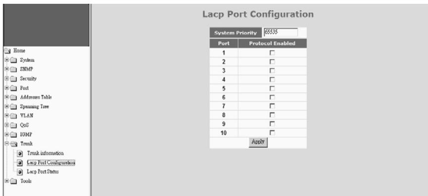
This page is used to configure LACP function. With LACP protocol, switches can learn trunk connections automatically.
