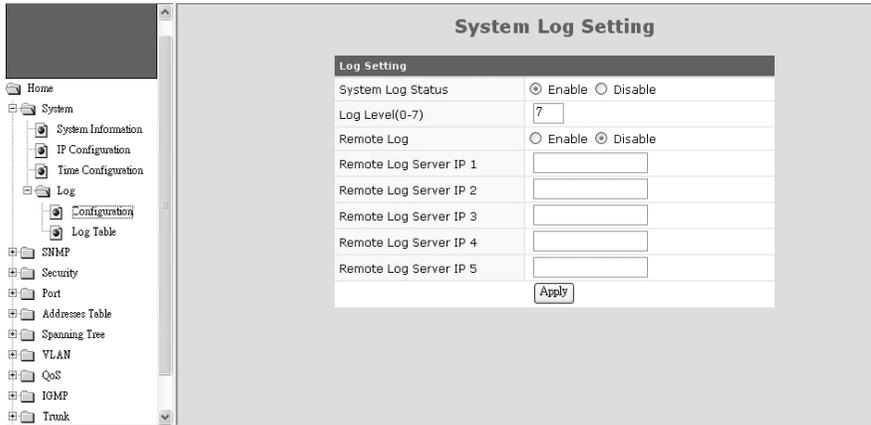
Users can configure System Log function and view log records here. If this function is enabled, the switch will record events to a log file and put the log file to flash.
