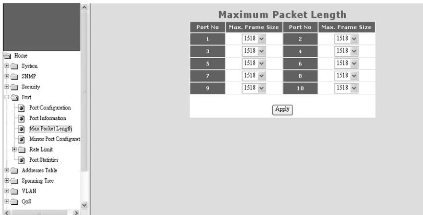
This switch supports Jumbo Frame function. And the maximum packet size could be up to 9600 byte/packet. You can select the maximum packet size for each port here.
