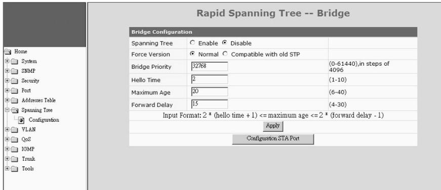
Here are the parameters for Spanning Tree operation on the switch.
