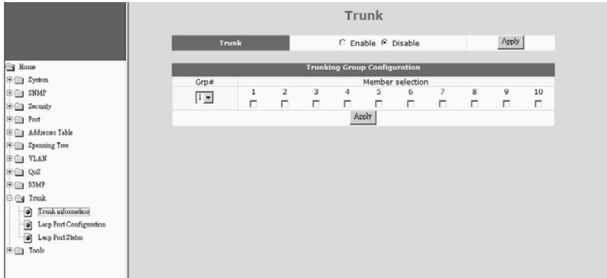
This table is used to assign ports to Trunk groups statically.
