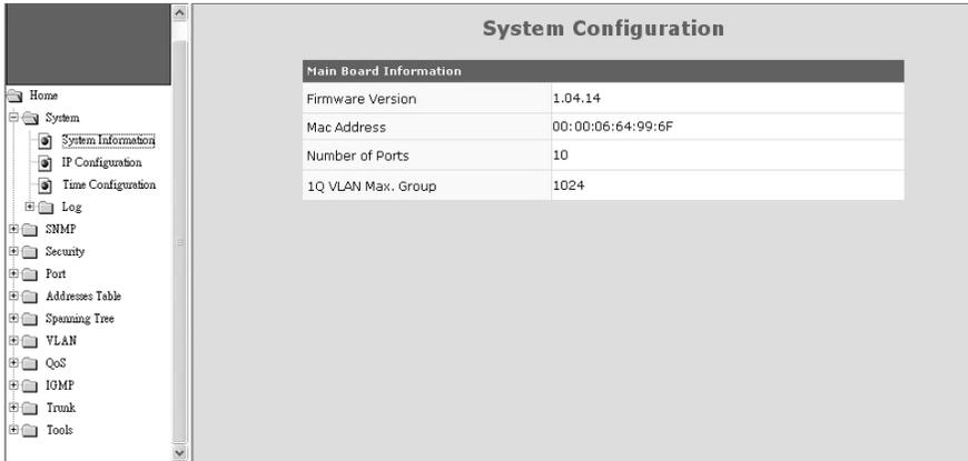
This function lists the system information about the switch. You can find the firmware version, Mac address, connection port number, and maximum VLAN group number here.
