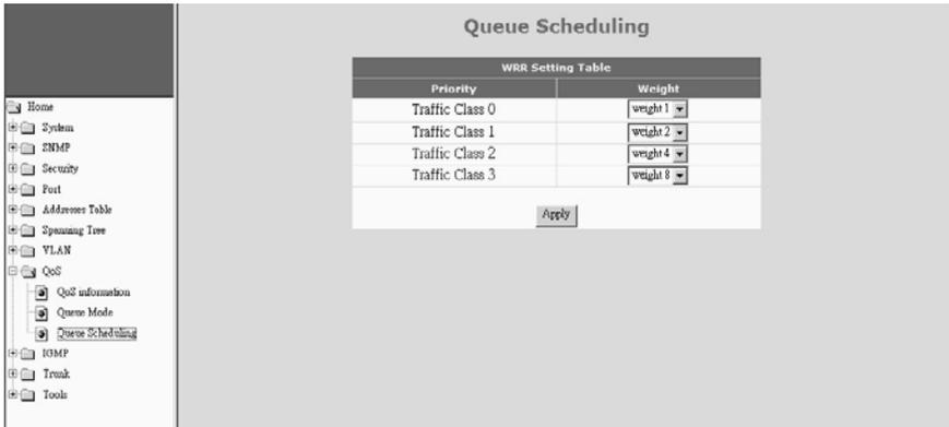
This function is used to configured the weighting of priority queues for WRR operation. And the output bandwidth will be shared with the ratio of weighting between priority queues.
