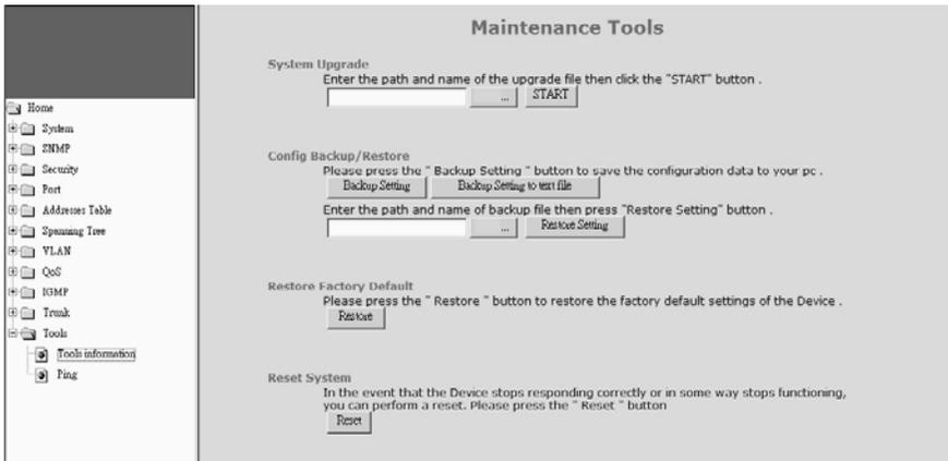
**System Upgrade :** This function will upgrade the system operation software from the web management PC.
