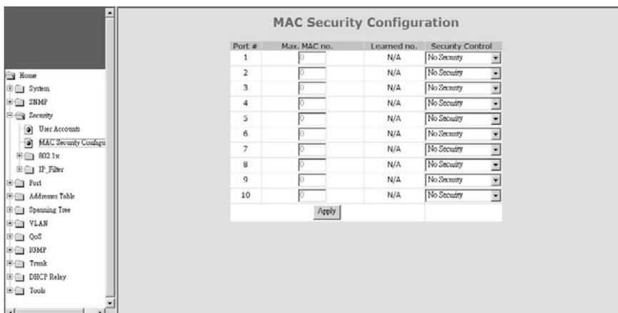
There are two Mac ID security modes for the switch. One is Static Mac ID Filter on Port, another is Dynamic Mac ID Number Limit on Port.
