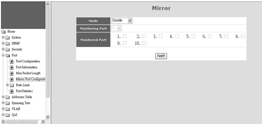
**Mode:** This is used to enable/disable Mirror function.
