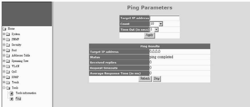
This function is used to ping network devices from the switch. It can be used to verify network connection.
