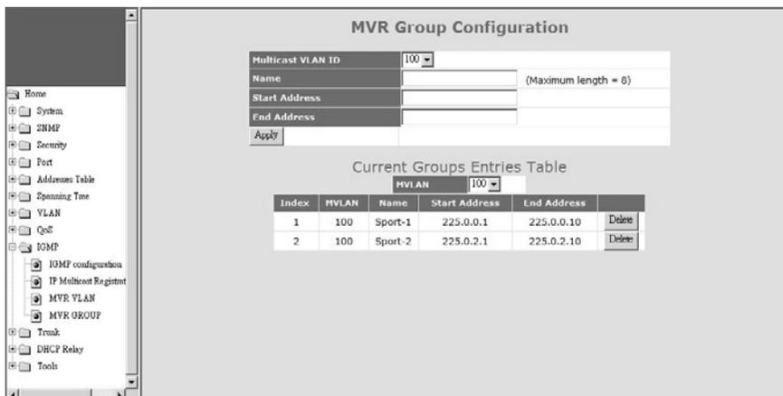
After the MVR VLAN is configured, you can assign IP multicast groups (video channels) to the MVR VLAN in “MVR Group” page. You can assign more than one IP multicast groups (video channels) to one MVR VLAN.
