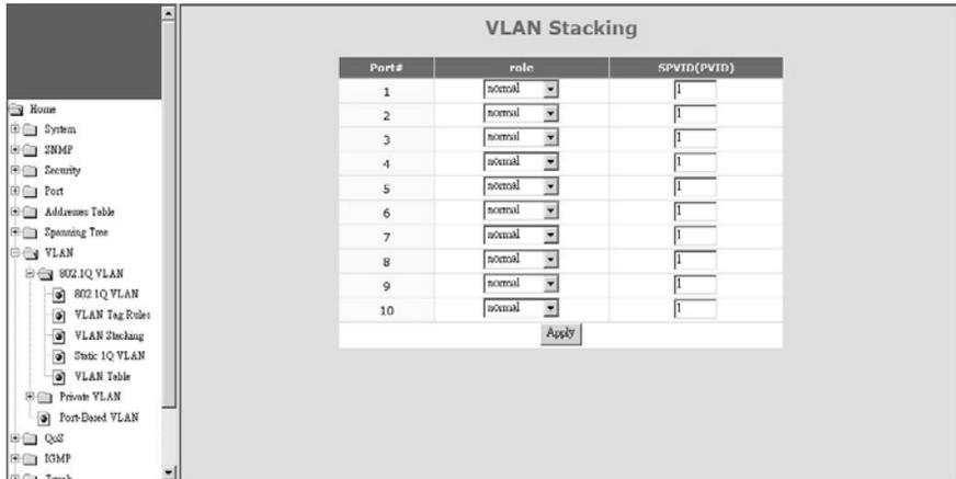
VLAN Stacking function allows two VLAN tags in a packet for 802.1Q VLAN tunnelling application through a central network.
