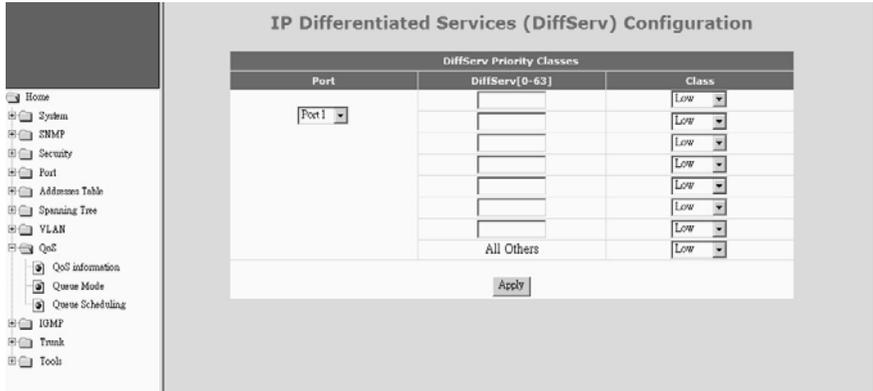
DSCP priority operation will use the priority setting in ToS field of IP packets for QoS operation.
