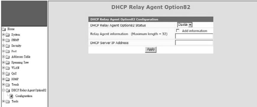
DHCP Relay function will control DHCP requests and forward DHCP requests to the assigned DHCP server. DHCP Relay Agent Option 82 function will add connection port, VLAN ID and switch information to DHCP requests and then send to the specified DHCP server. Based on those information, DHCP server will assign an IP configuration in the DHCP reply. This is a security function.
