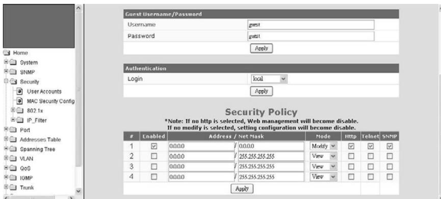
This is used to setup the IP addresses that can manage this switch. They have different access rights set in “Mode”. And the remote management interfaces (Http/Telnet/SNMP) could be enable/disable for different administrators. This function is for security policy of switch management.
