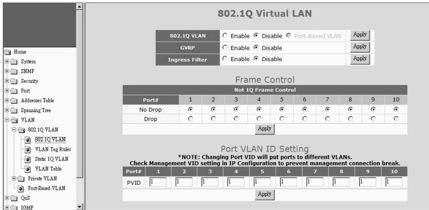
**802.1Q VLAN** : This is used to enable/disable 802.1Q VLAN function.
