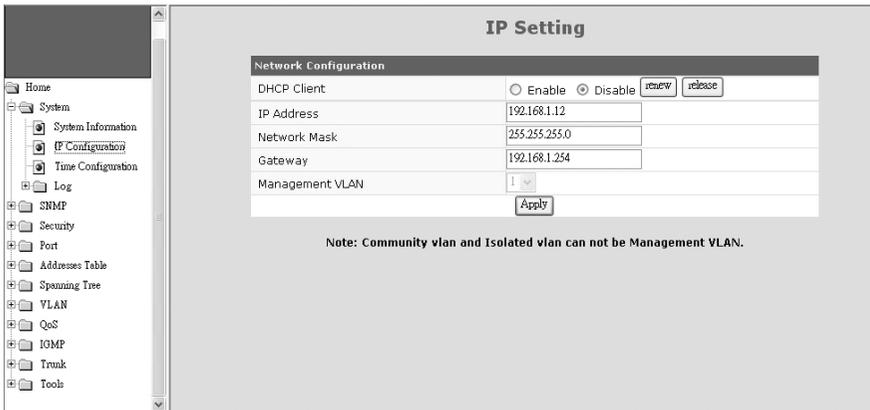
This function is used to setup IP configuration of the switch. You can enable DHCP client function to get IP configuration from DHCP server
