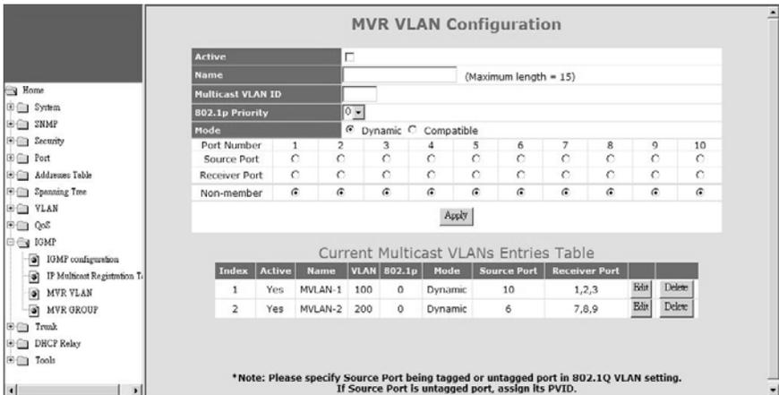
This page is used to configure MVR (Multicast VLAN Registration) function. VLAN function will isolate traffic between VLAN groups. But it will also isolate IP multicast traffic for subscribers in different VLANs. The MVR function allows one multicast VLAN to be shared by subscribers in different VLANs. That can reduce the multicast traffic for VLANs.
