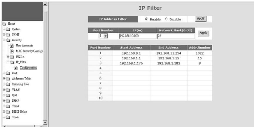
Because it is a subnet specified by IP address/Network ID Number(0~32, or called Subnet Mask), the start IP address, end IP address and allowed IP address number are shown in the table.
