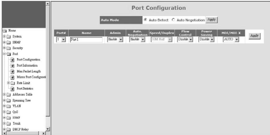
This function is used to configure port settings of the switch. You can enable/disable a port, set it to fixed 10M or 100M or 1000M ... and so on.
