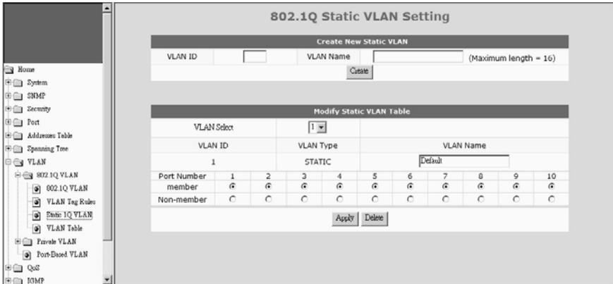
This function is used to maintain 802.1Q static VLAN.
