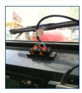
1. Prepare 3 wires form car harness then connect power cable attached to device.
