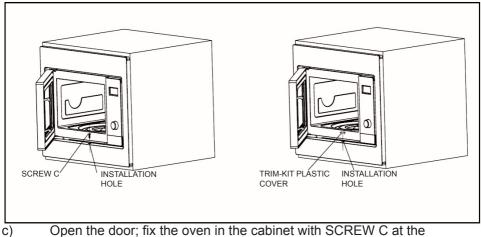
INSTALLATION HOLE of TRIM KIT. Then fix the TRIM-KIT PLASTIC COVER to the INSTALLATION HOLE.
