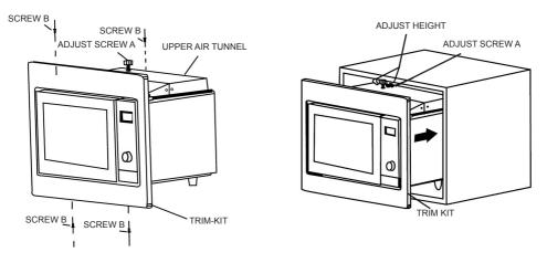
b) Fix ADJSUT SCREW A on the UPPER AIR TUNNEL of the oven, and fix the TRIM KIT with SCREW B. Then install the oven into the cabinet. Make sure that the upper side gap between the TRIM KIT and the oven is the same as the bottom side.
