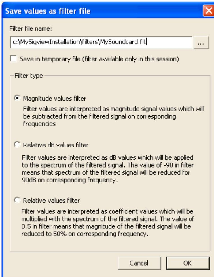
7. You can use this saved filter for any data analysis using sound card signal to correct your measurement and remove artifacts caused by the sound card imperfection. To do so, go to your data acquisition signal from step 1 and apply "Signal tools/Filter..." menu option on it. In the dialog, choose your saved MySoundcard.flt filter. It means that we remove from the signal exactly the frequency components introduced by the sound card:
