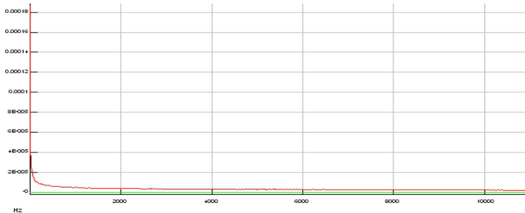
5. This curve is characteristic frequency response of your sound card. Normally, this curve is shown on log scale, but we need it like this so we can convert it to a Custom Filter curve. As a next step, go to Averager window and choose "File/Save as filter curve" option from a menu.
