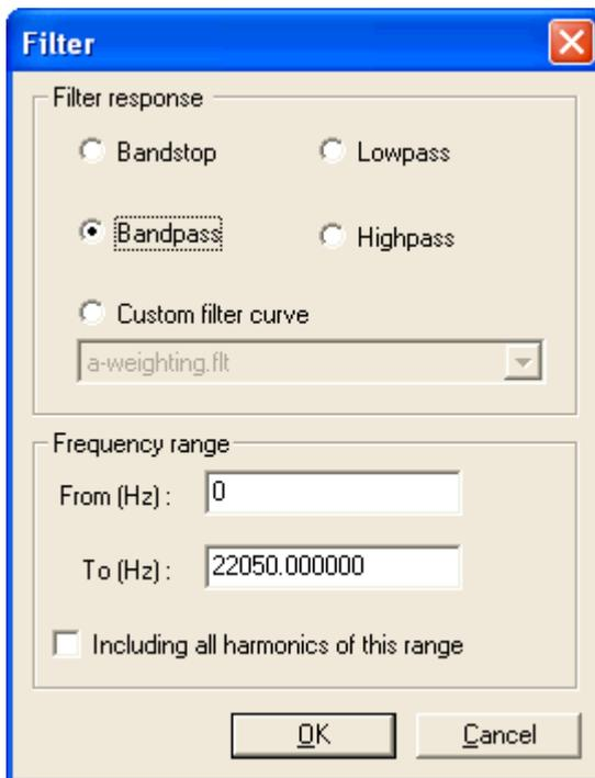
*SIGVIEW* uses FFT-based filtering algorithm. It is a combination of the FFT calculation, changes in the FFT result (filling some frequency bands with zeros or applying custom filter curve) and the inverse FFT calculation. This method is relatively slow compared to other filtering methods, but is usually very accurate.
