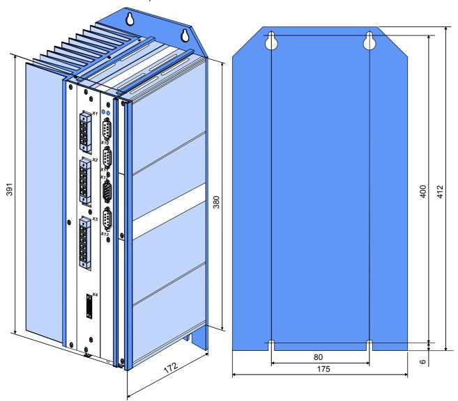
Compax3 S300 V4 is force-ventilated via a fan integrated into the heat dissipator!
