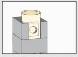
16. Place the block using grout. Put pipe glue on the bottom part of the pipe and place it on the tee. Next, place the stabilising rings.
