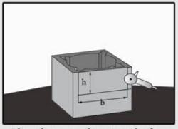
1.Place damp-insulation on the foundation. Remember to consider the "0" level. Use a grinder to cut an opening (h=12cm, b=22cm) in the top part of the first block..
