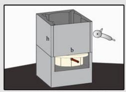
3.Before placing the second block, cut an opening size h=26cm (attention: the block hight is 24cm, the remaining part should be cut from the next block), b=26cm. Place the block on the first block using grout.
