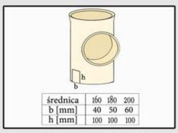
5.Cut a pressure equalizing opening (size b x h) in the bottom of the inspection tee.
