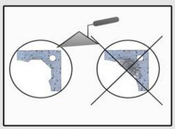
4.Remember not to block the air-channels when putting grout.
