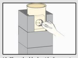
13. Place the block with the opening and a pipe without glue and grout. Next, using the connection frame, mark a place for connection opening in the pipe.
