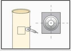
14. Remove the block and the pipe. Cut an opening according to the drawn dimensions and glue the connection branch into the pipe.
