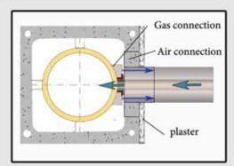
15. Use pipe glue to paste the connection branch into the pipe. Use grout to paste the outer air connection element into the block, centering it towards the gas connection branch.
