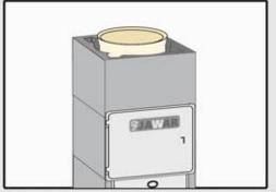
10. Next, place the chimney door and the condensate tray cover. Installation of the chimney door can be also made after building the whole chimney.
