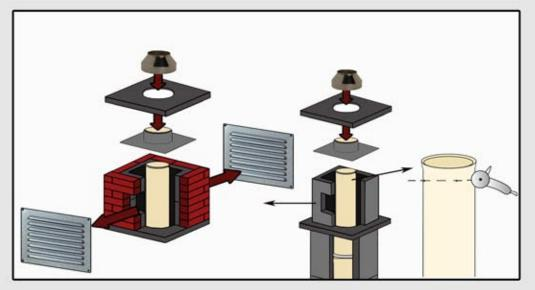
Cut two opposite openings size 17x20cm for ventilation checks in the last block. Place the block using grout. Next, place the covering plate. Remember to center the opening towards the pipe.
