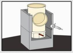
7.Put glue on the cleaned, moistured edge of the condensate tray. Next, place the tee and center it exactly.
