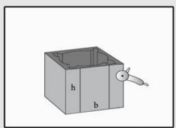
12. Cut on opening size h=24cm, b=20cm in a block for the gas connection.
