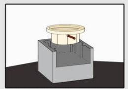
2.Place the first block and fill it with concrete up to the opening. After the concrete has set, put the condensate tray into it, front towards the opening.
