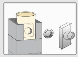
17. After the pipe glue has set, insert gas membrane into the connection branch. In case of 2 connections on one storey, the hight difference between the connections' axes should be at least 30cm.
