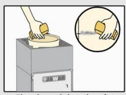
11. Place the needed number of pipes and blocks until the demanded connection hight is reached. Remove the excessive pipe glue using a moist sponge.
