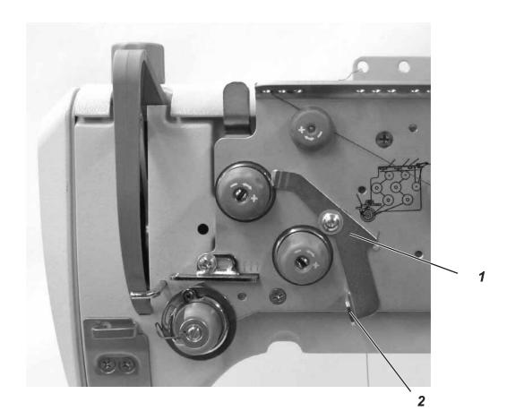
The supplementary tension is being switched on and off with lever 1.
