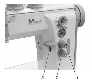
The special sewing machines 868 are, depending on the subclass, equipped with two setting wheels. Thus, two different stitch lengths can be sewn, that are activated by actuating a key (see chapter 6.17).
