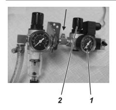
To set the contact pressure pull out the turning handle 2 of the pressure regulating valve of the seam center guide and turn it.
