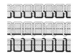
Fig. A: Correct thread interlacing in the center of the material
