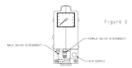
2. CONVERSION OF TOOL: DISCONNECT TOOL FROM AIR SUPPLY. REMOVE PLUG, AND REPLACE WITH FEMALE QUICK DISCONNECT AT LOCATION SHOWN IN FIGURE 2. SCREW MALE QUICK DISCONNECT INTO REMAINING TAPPED HOLE. BE SURE TO INSTALL FEMALE QUICK DISCONNECT WITH KNURLED SLEEVE IN TAPPED HOLE NEXT TO AIR SUPPLY LINE.
