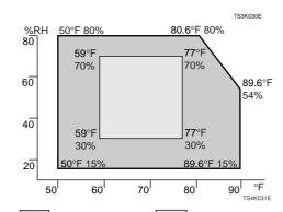
Possible operation range Recommended range The machine must be level within 5 mm, 0.2" both front to rear and left to right.
