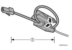
Attach the network interface cable to the jack on the board.
