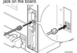
Connect the other end of the network interface cable to the network.
