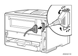
Attach the other end of the interface cable to the interface connector of the computer. Secure the cable.
