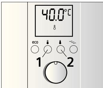
Desired temperature button **1** is preset to 40°C, desired temperature button **2** is preset to 60°C.
