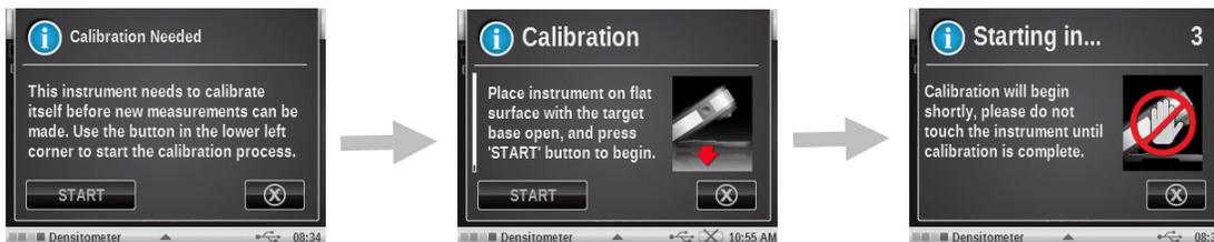
A calibration is also required when the Measurement Condition switch is changed and calibration has not been performed, or has timed out for that position. In this case, tap the START button on the screen to begin the procedure and follow the remaining screen prompts.
