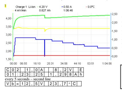
Charging ends when threshold voltage is detected and simultaneously charging current is decreased. When *Fast* mode is on charging current is controlled with pulses, which makes it possible to reduce charging time more than two times.
