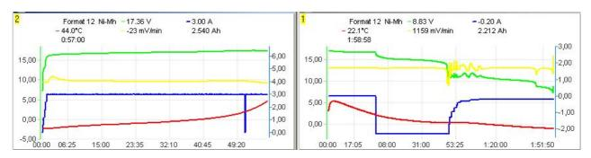
Formatting a battery means to perform demanded number (1 to 8) of discharging-charging cycles. Discharging is performed in Auto mode until threshold voltage is reached, which depends of cell type. Reconditioning a battery – special formatting mode which allows to repair the battery.
