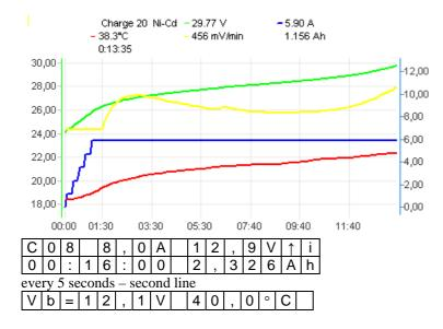
Charging ends when voltage drop  $(-\Delta v)$  or inflex point is detected.
