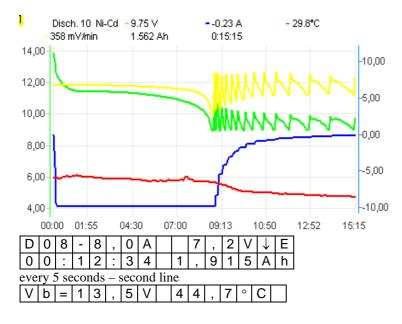
Discharging lasts until battery voltage reaches threshold voltage for given cell type. In *Auto* mode current is decreased by ½ each time the threshold voltage is reached. Discharging process ends when discharging current is less than 200mA.
