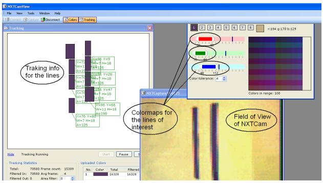
In line tracking mode, beginning point and end point coordinates of a line representing the object are returned. In the following picture, the bounding boxes are drawn for the line coordinates received from NXTcam:
