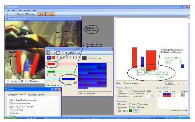
The top left window in the picture below shows the field of view of NXTCam. The objects of interest from this view are the red and blue pens. In the object tracking mode, the bounding box coordinates are returned, as shown:
