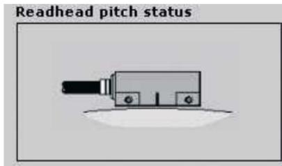
**Figure 5:** Optimum pitch installation has been achieved.
