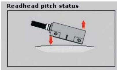
**Figure 3:** The cable end of the readhead is set too high and needs to be adjusted as shown by the arrows in the diagram.
