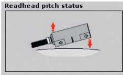
**Figure 4:** The cable end of the readhead is set too low and needs to be adjusted as shown by the arrows in the diagram.
