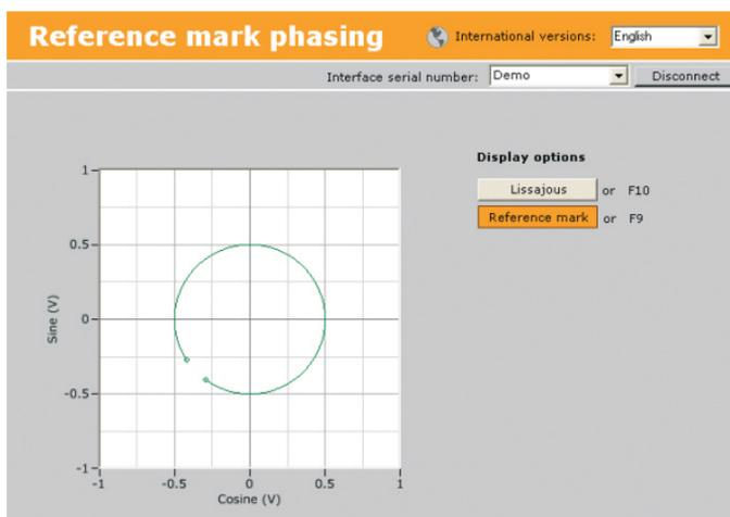
**Figure 7: Reference mark phasing screen**
