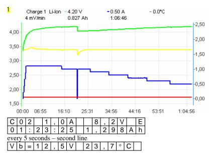
Charging ends when threshold voltage is detected and simultaneously charging current is decreased. When *Fast* mode is on charging current is controlled with pulses, which makes it possible to reduce charging time more than two times. Current limitation can occur when voltage overstep maximal value for given cell types. We recommend the *Pulsar EQUAL* <u>Equalizer from ELPROG</u>.
