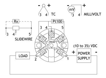
\* Fit Rx for all potentiometers with end to end resistance > 390  $\Omega$ . Such that total end to end resistance is > 200  $\Omega$  < 390  $\Omega$ .
