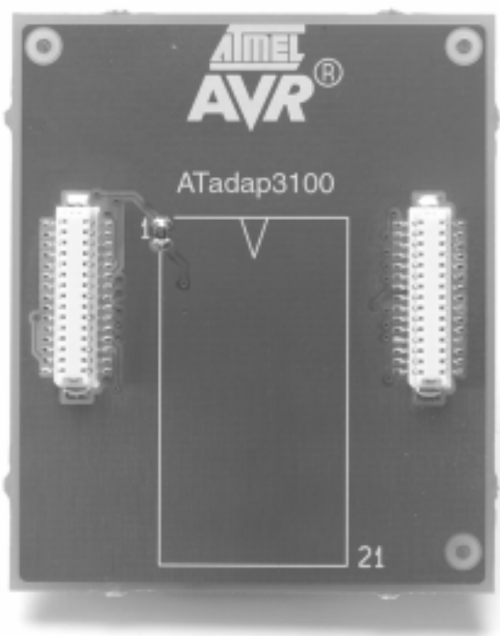
Figure 4-5. Personality Adapter for AT90S8535/4434 – ATadap3100
