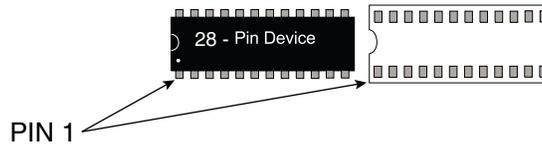
There is another method of checking that the device is inserted the right way and that is to check the notches on both the device and the programming socket. At the end of the device a notch is cut out. There is also a notch cut out on the device socket, which is also printed on the board. The notch on the device must correspond with the notch in the socket.
