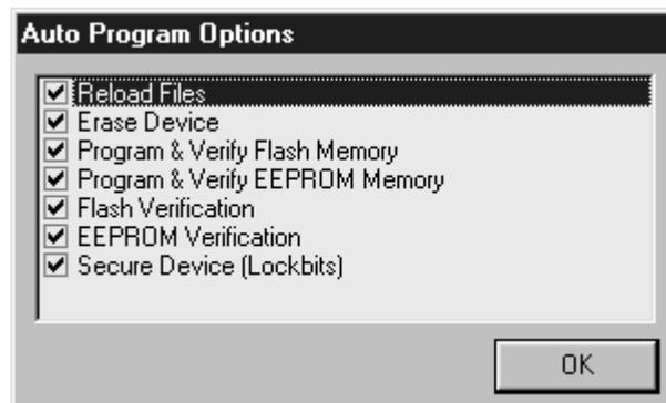
Check the operations required (v = on) and all the chosen operations will be carried out when Auto Program (F5) is used. If “Program Fuses” is checked, then another dialog box will appear, after this list is closed, where the device-specific fuses can be set.
