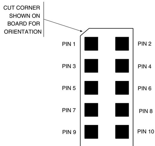
**Figure 4-6.** 8-pin Connector
