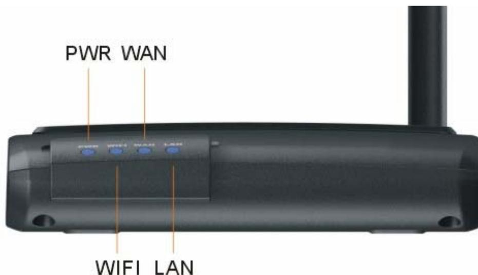
The Gateway's LEDs are located on the front panel(View from left to right).
