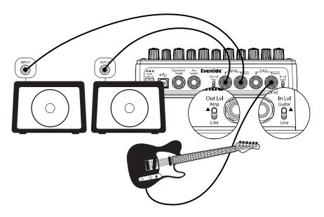
Connect your guitar cable to ModFactor Input 1 and a cable from ModFactor Output 1 to one amp and a second cable from ModFactor Output 2 to the other amp. Input Level switch (In LvI) should be set to GUITAR and Output Level switch (Out LvI) set to AMP.
