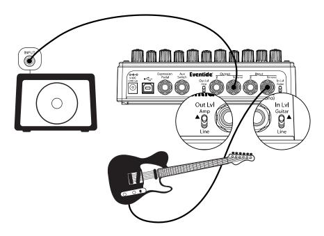
This is the simplest way to connect ModFactor. Connect your guitar cable to ModFactor Input 1 and a cable from ModFactor Output 1 to your amp. Input and Output Level switches (In Lvl & Out Lvl) should be set to GUITAR and AMP.
