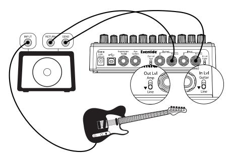
If your Amp has an Effect Loop, you can connect ModFactor's Input to the Amp Effect Loop Send and ModFactor's Output to the Amp Effect Loop Return. Most guitar amp's Effects Loop run at Line Level so set ModFactor's Input and Output Level Switches to "Line."
