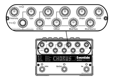
ModFactor uses 2 LFO's (Low Frequency Oscillators) to create classic or FM/AM modulated versions of many popular modulation effects. The primary LFO drives the main effect and is controlled by the three top row controls, **Depth**, **Speed** and **Shape**.
