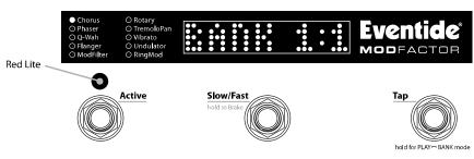
Note: The 40 Presets can be based on any of the Effects. You can choose to have all 40 presets based on Chorus. Or, two based on Chorus, three based on Flanger, five based on Vibrato, etc. - or any combination.
