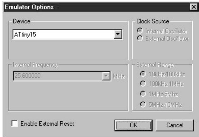
**2.2.1 Device** Select the device from the list. The device list includes all devices currently supported in the emulator.
