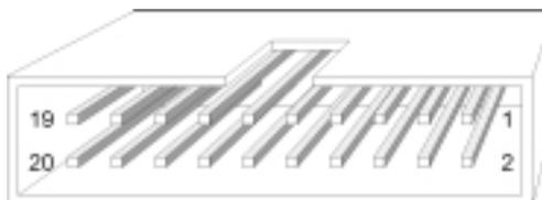
The connector marked **LOGIC ANALYZER 2** on the back panel of the AVR ICE unit has the following pinout with signals from the instruction data bus.
