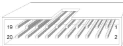
The connector marked **AUX** on the back panel of the AVR ICE unit is used for external triggers and has the following pinout.
