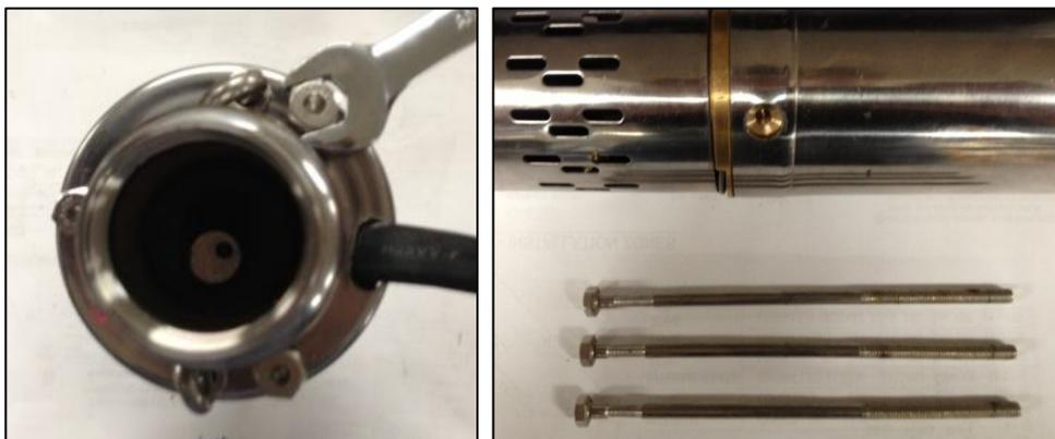
Step 3 Gently pull apart the pump outlet, shroud and motor ensuring that the power cable is not damaged.
