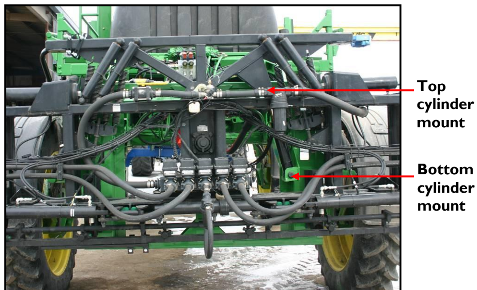
Figure 18: Roll Cylinder Mounts
