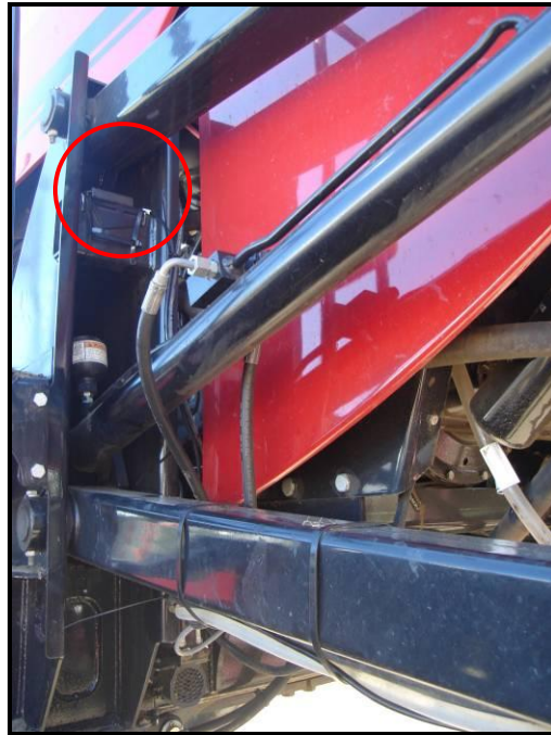
Figure 39: Example of Reference Frame Roll Sensor Mounting
