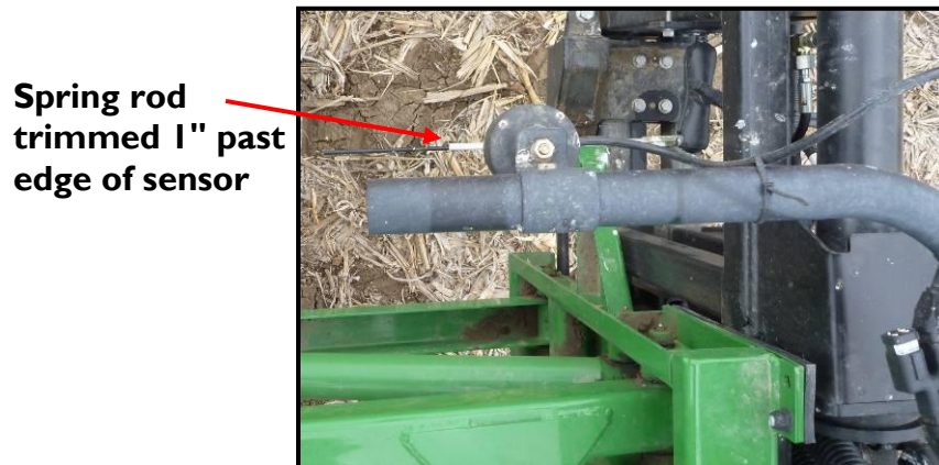
Figure 42: Active Roll™ Sensor and Rod Alignment
