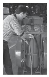
Lay hose straight on ground to its full 50' length. Start first regular loop counter-clockwise by placing it over the top bracket and between the side brackets as shown.
