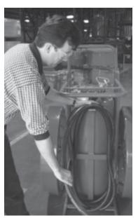
The next loop is a regular "hose in front" loop. Succeeding loops are alternated, reverse, front, etc. until the full six loops are installed.
