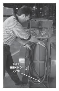
The second loop is a "reverse" loop. Note that the hose passes behind the loop on this reverse coil.
