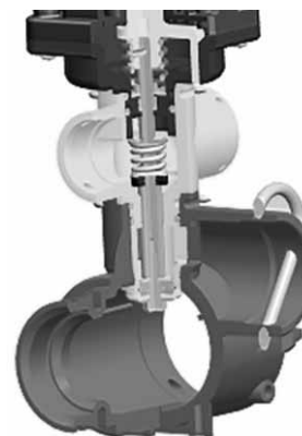
Picture 25 EFC without the equalization on the valve
