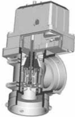
Figure 4 Pressure regulation valve with its duty circle
